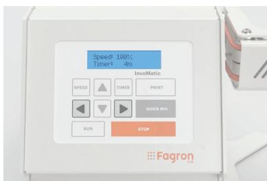
1. With the mixer in the stationary position, press and hold the "**LEFT**" and "**RIGHT**" buttons.
