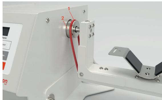
3. To fit the inversion arm, place the orange belt (1) over the pulley (2).
