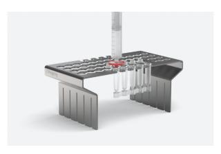
**3.** Fill the FagronLab<sup>™</sup> Monodose with the eyedrop solution.
