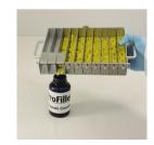
**4.** Open individual gates (push to left) and tilt Counter to transfer capsules into a bottle.
