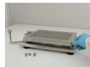
3. Unscrew 4 thumbscrews from corners of Filler Base.
